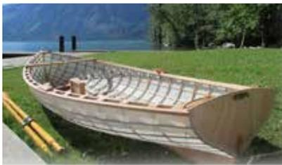
◀ **12' Geodesic Sailing Dinghy. A poly-tarp sail sprit-rig with well built fir spars**
