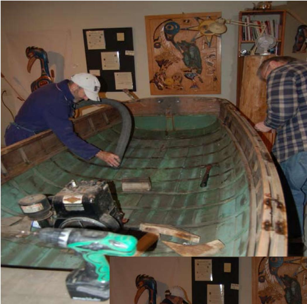
Ian Douglas and Dave Knott preparing the hull prior to replacement of ribs.
